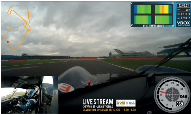
Front right tyre hotter in the middle
