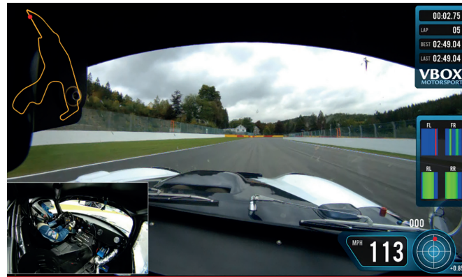
Front right tyre colder in the middle
