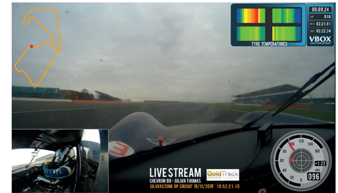
Front left tyre showing steep temperature gradient of 23°C
