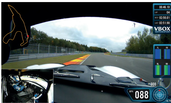
Too much rear bias leads to cold front tyres during turn in
